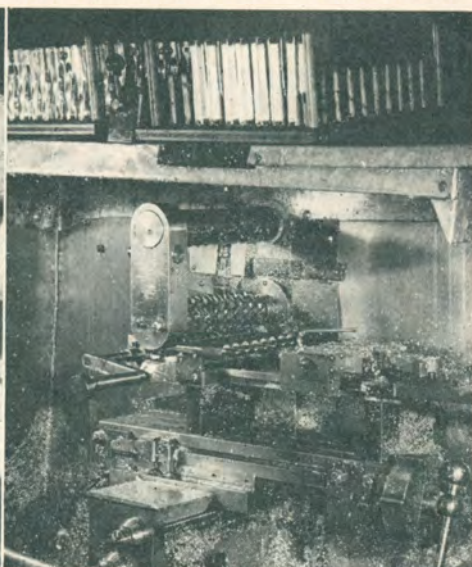
Left above, hollow rings or gaskets are being cut from sheets of Koroseal. Center, eight milling cutters may be seen among duraluminum flakes on this 90% electrically automatic pipe making machine. Right, the plunger assembly is polished.
