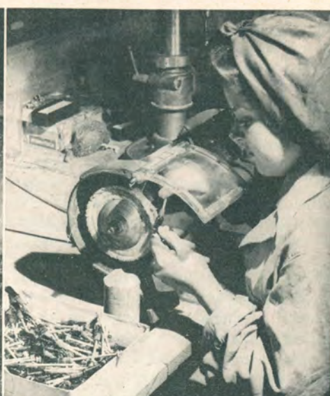
Left above, hollow rings or gaskets are being cut from sheets of Koroseal. Center, eight milling cutters may be seen among duraluminum flakes on this 90% electrically automatic pipe making machine. Right, the plunger assembly is polished.
