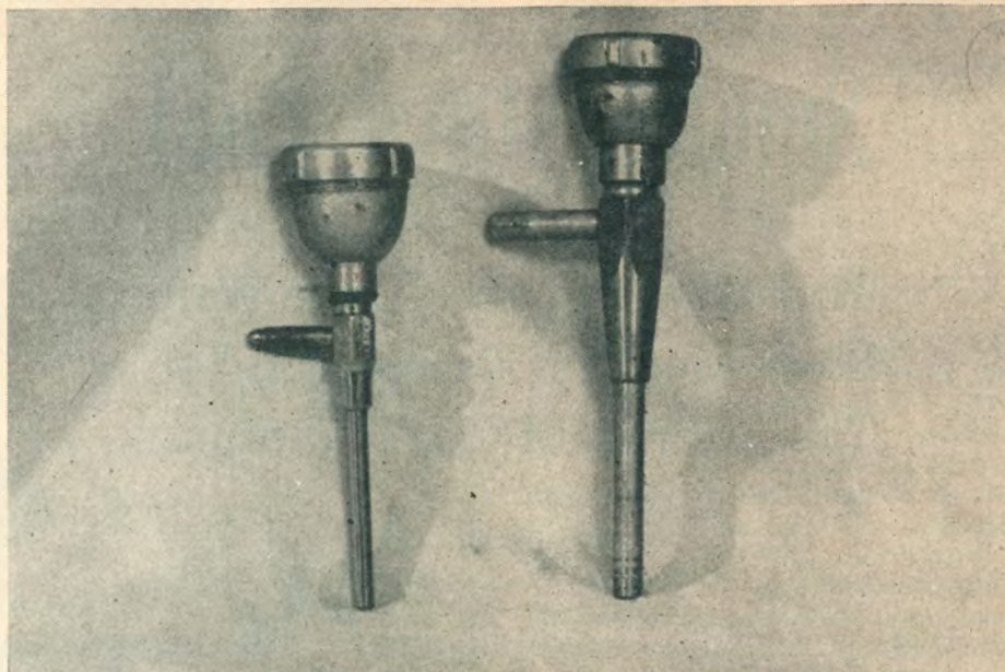
The filter pumps used in the device are available in several sizes, two of which are shown here. In the article the author describes the advantages of each one.
