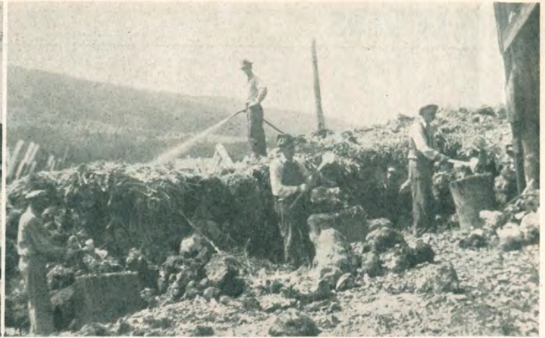
Left, comparative size of the Carolina briar burls is shown after being removed from the ground. Right, they are then covered with sugar cane stalks and watered in order to prevent their drying out before they are sawed into small blocks.
