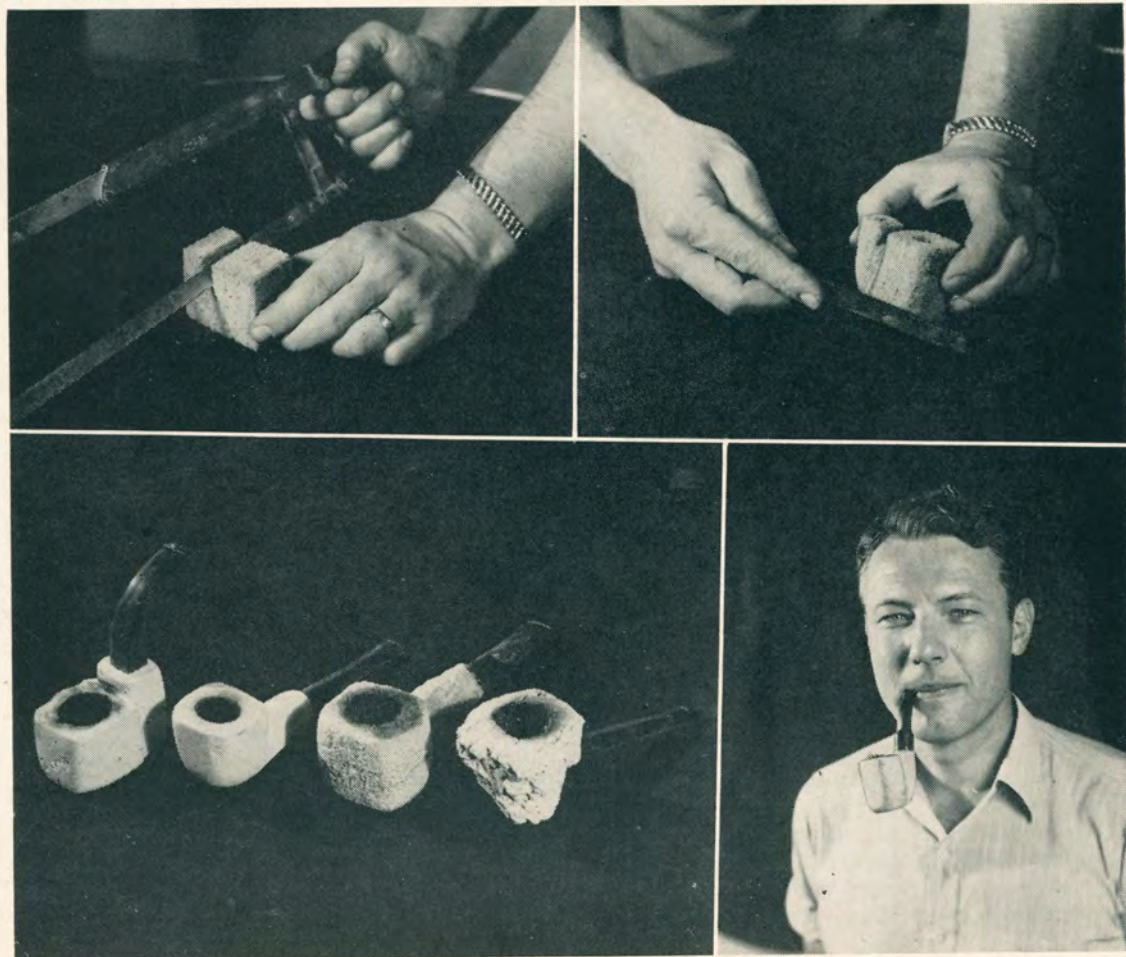
Upper photos illustrate how block of pumice is first cut to shape with a hack saw and then finished with a file. Below, left, some of the many pipes made of pumice by the author, right.
