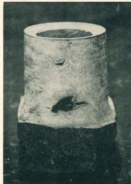
The outside of this block was smooth, but inside a flaw made the block useless.
