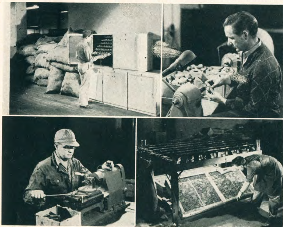
Left, above, heat treating bowls to shorten break-in period. Right, hand carving the bowl. Left, below, making the stems; right, briar getting infra red treatment.
