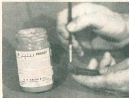
Top, broken stem is removed with the aid of a screw. Center, heated stem is bent to any desired shape. Bottom, thin coating of shellac fixes loose fitting stem.
