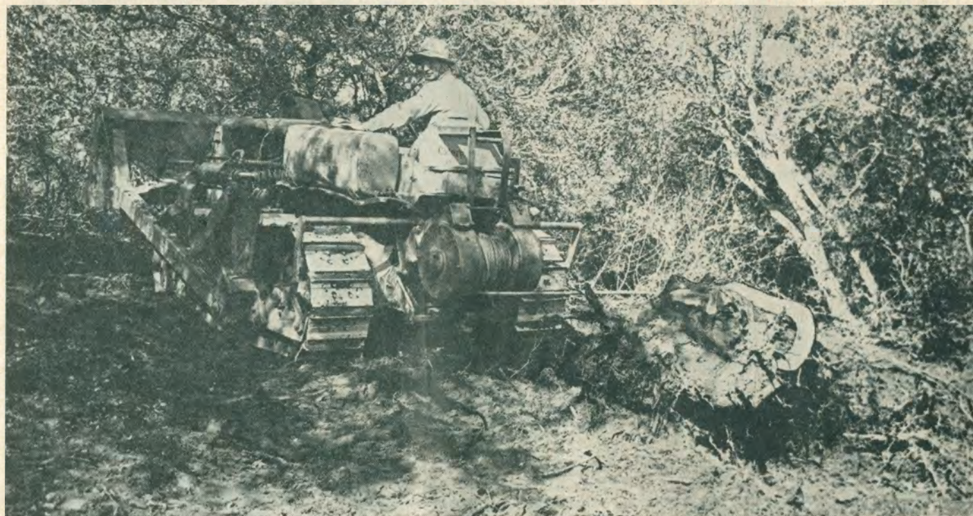
This is one of the big Caterpillar bulldozers used in digging out Mission briar burls which will eventually be made into smoking pipes. Both the dozer shovel and the winch at the rear of the "cat" are used to dig the burls out of the ground.
