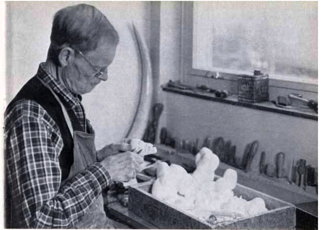
Genuine meerschaum pipes are cut by hand — today as 200 years ago. Here is Lars Prestmoen making a pipe bowl.
