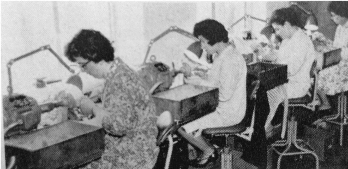
Woman operators sanding bowls to remove waste and retain exact shape
